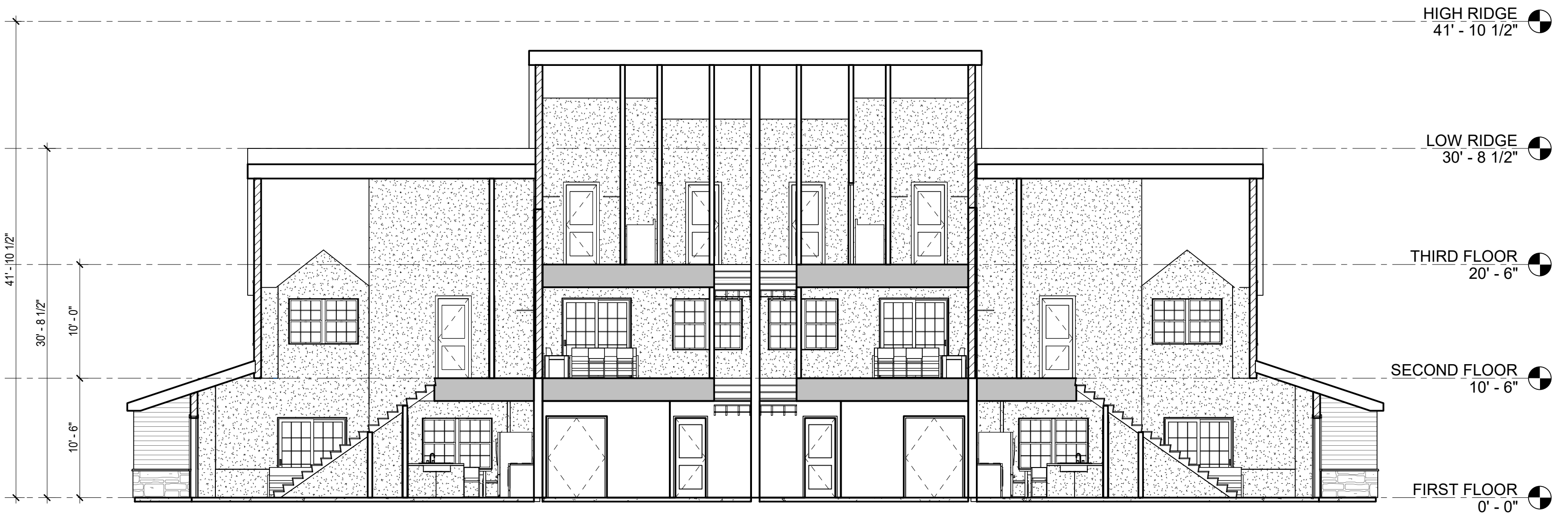
BUILDING SECTION 01 - TYPE A SCALE: 1/8" = 1'-0" 1
