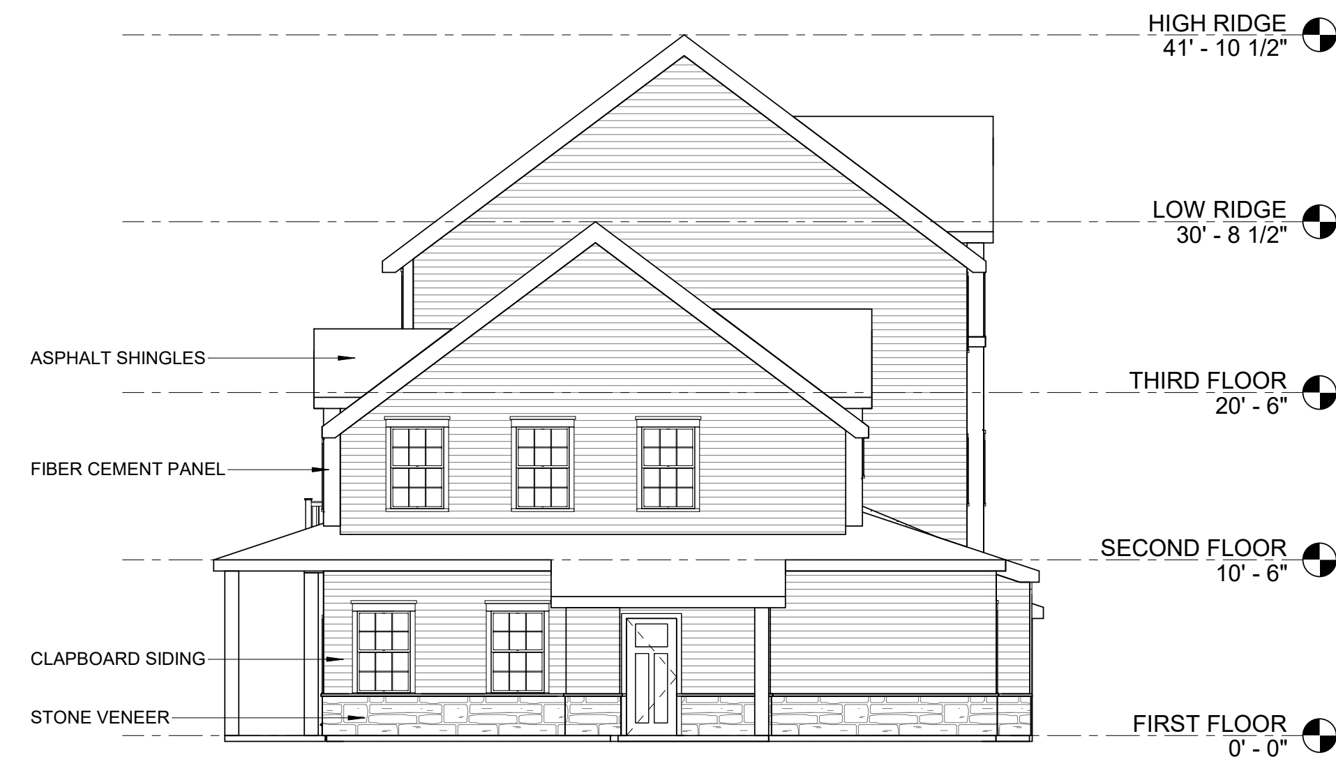
WEST ELEVATION - TYPE A
